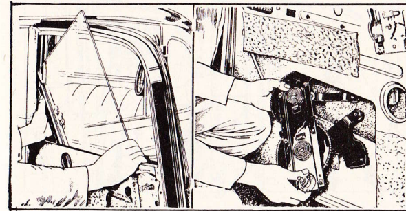
Fig. 238.—How To Remove Glass and Regulator Mechanism From Ford V8 Doors.
